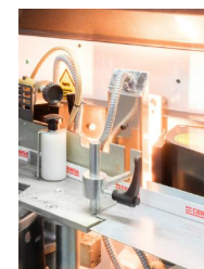
Infrared lamp at entrance & before pressure zone
