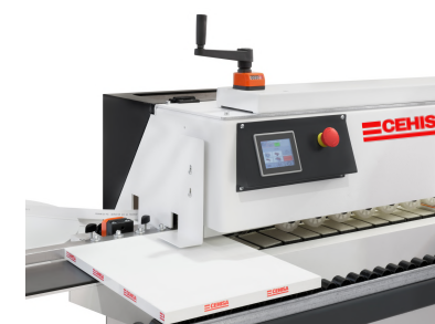
Handy regulation of the pressure beam
