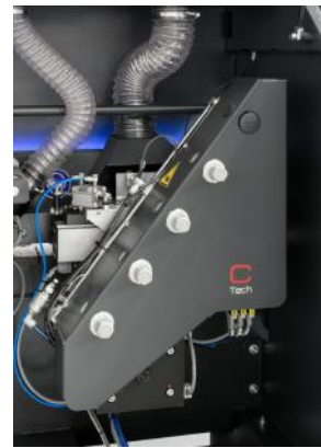
2 motors pneumatic tilting End trim
