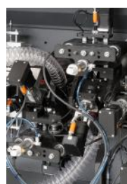
Radius Scraper station w/ Multi- radius tooling
