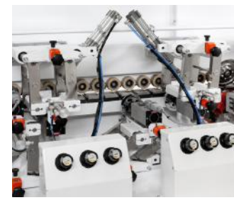
4 motors Corner Rounding station
