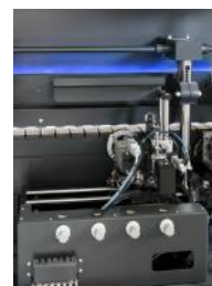
Corner Rounding station w/ Motorized adjustment
