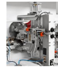
High speed Radius Scraper station
